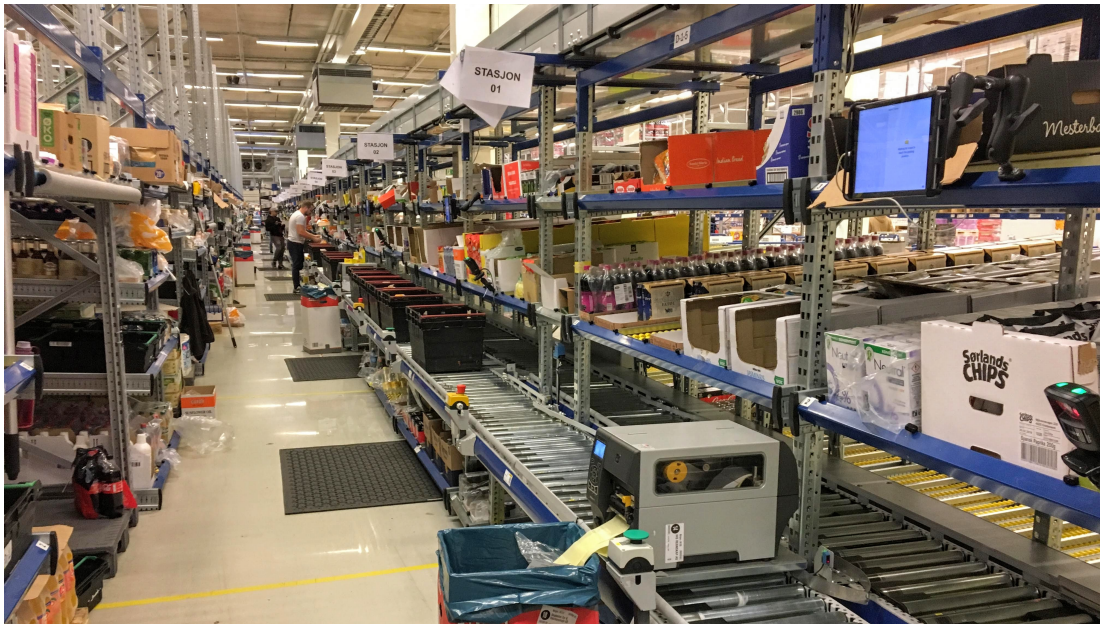
Figure 2.3: This figure shows the stations along the assembly line in the dry stock section of the warehouse. There are 13 stations down this aisle. The belt furthest on the right is the main line. The belt second most to the right is the box positions for the stations.
